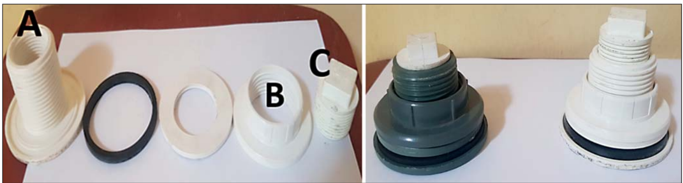
Figure 1 - A polyvinyl chloride plastisol main T09 Male Adaptor plumbing device modified into a rumen cannula and demonstrating its various components for rumen cannulation. A: Plastic hose with inner flange. B: Plastic outer flange and screw. C: Stopper.
